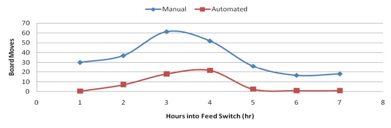
Console Operator Moves per Hour Comparison from paper "Improving Refinery Unit Transitions Using Process Automation Technology in a base Oil Hydroprocessing Facility. AIChE Spring 2011 Robert M. Tsai, Chevron, Richmond, CA
