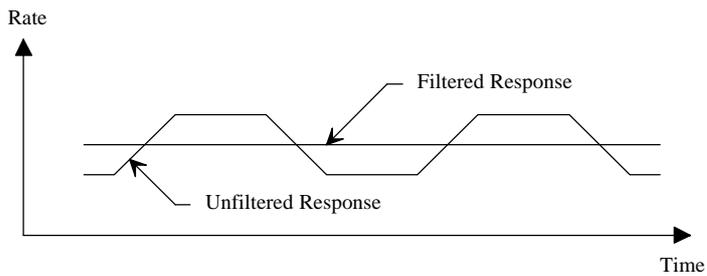
As a guideline to the degree of filtering to be used, the following table shows the response to a step change in input. The value, CAL 06, is the filter constant which is programmed during the Programming routine. The times for the display value to reach 90% and 99% of full swing are given in seconds, for different values of CAL 06.
