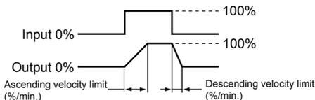
Setting range of velocity limit: 0.1 to 600.0%/min.; minimum unit is 0.1 %/min.
