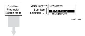
When zero adjustment function has been completed, the system returns automatically to the sub-item selection screen (D).
