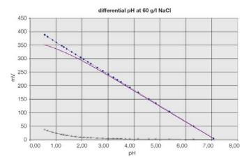
In this graph you can see that in this application the sensor behaves like any normal pH sensor with the Isopotential at 7 pH, 0 mV and a linear response over the complete pH range down to 2 pH. Below 2 pH we see a slight non linearity.
