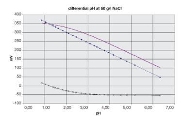
In this graph we see that the sensor is only linear down to 3 pH and the Isopotential value is now 8 pH or the Asymmetry Potential at 7 pH is + 60 mV.
