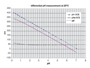
Now we see that the sensor output is linear over almost the complete pH range with only a slight loss of sensitivity below 1 pH. The Asymmetry Potential is now -50 mV at pH7, but
