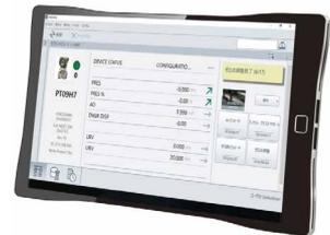
FieldMate is PC software that adjusts, configures, and manages various field devices in a plant. FieldMate R3.02, the latest version, has improved functions to help customers perform maintenance work efficiently. The new FieldMate reduces the time for loop tests by one third compared with the previous version.
