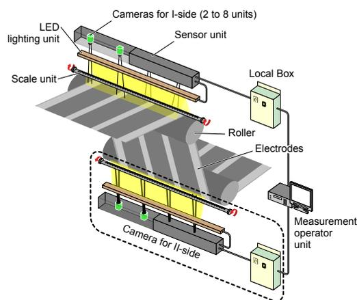
**Figure 2** System configuration for both sides measurement
