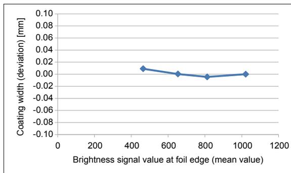
**Figure 5** Error due to brightness fluctuation
