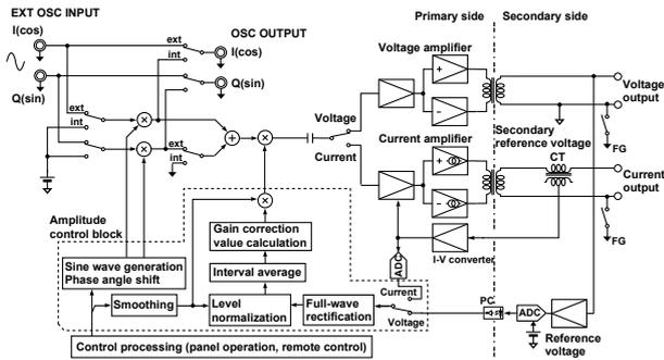
Figure 3 Block diagram of 2558A
