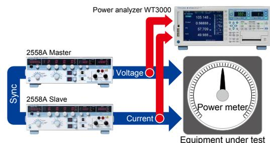
Figure 2 Example of a connection configuration for synchronized operation
