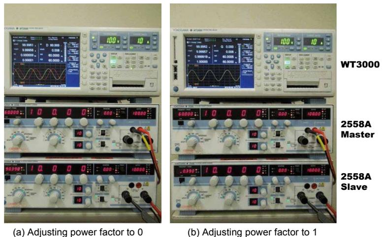
Figure 7 Example of a power calibration system composed of the two 2558A and WT3000
