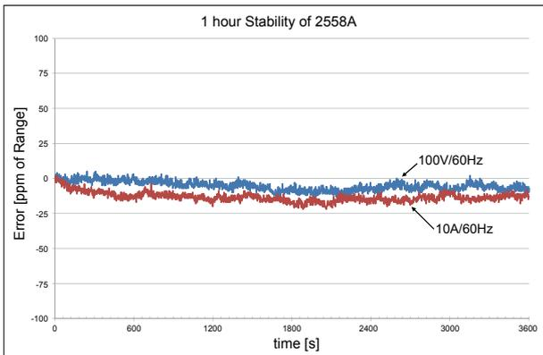
Figure 5 Measured stability in one hour
