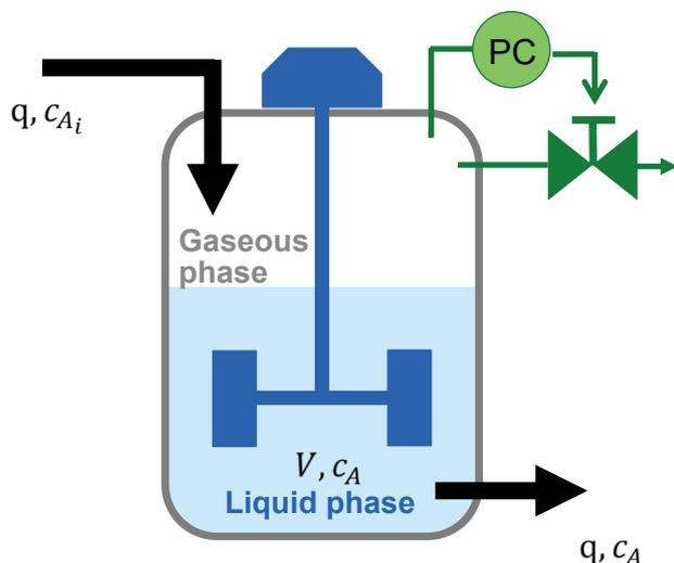
**Figure 4** A continuous stirred reactor tank
