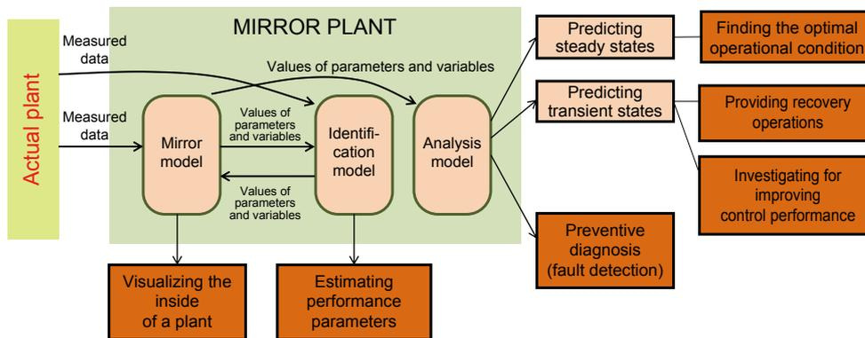
**Figure 1** Configuration of MIRROR PLANT
