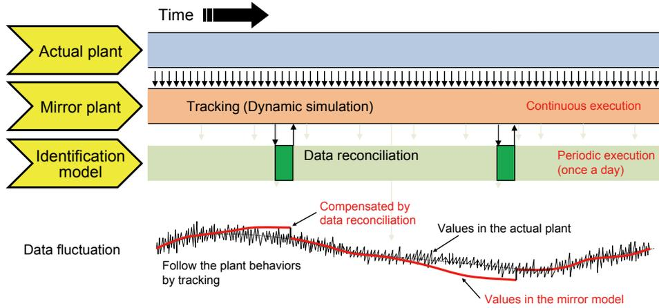
**Figure 3** Operation sequence of MIRROR PLANT
