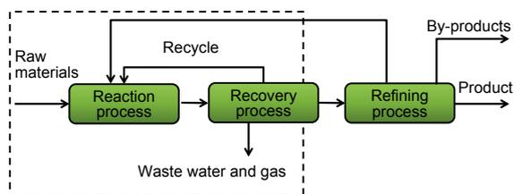
**Figure 5** Basic structure of a chemical process
