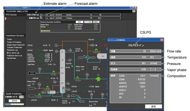
**Figure 2** An example of an operational assistance screen of MIRROR PLANT
