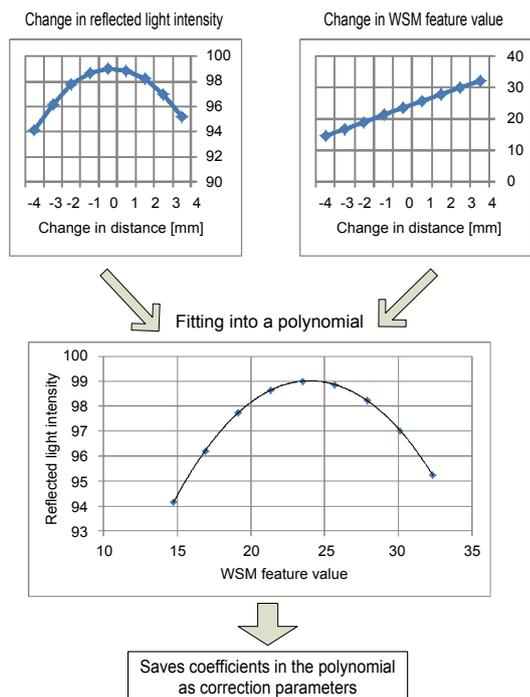
**Figure 7** Determining correction coefficients used for the WSM
