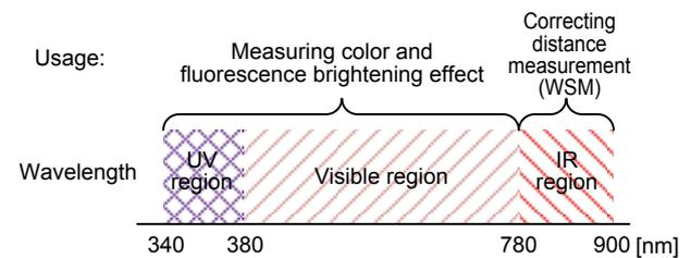
**Figure 6** Application of each wavelength region in the optical spectrum
