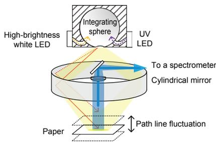
**Figure 3** Conceptual diagram of the optical system
