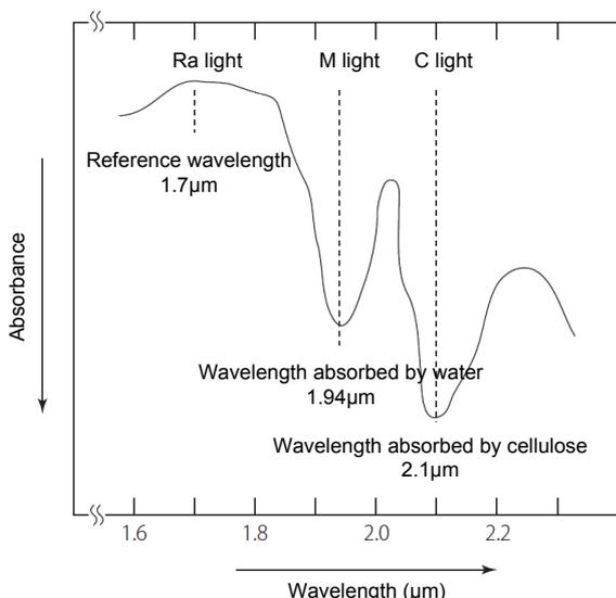
Figure 2 Typical absorbance in the near infrared region
