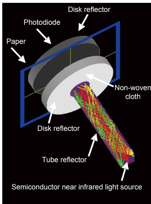
Figure 3 Optical system of the new moisture sensor
