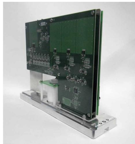
Figure 1 External view of the moisture sensor
