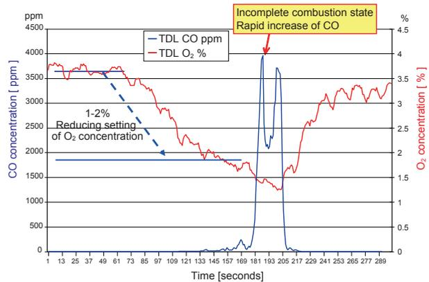
**Figure 4** O<sub>2</sub> and CO Concentration Changes in a combustion furnace at Low Oxygen Concentration Operation
