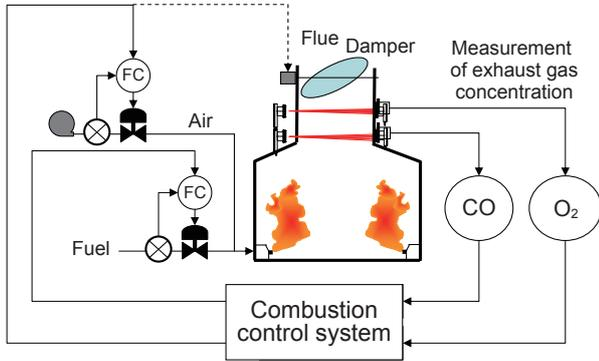
Figure 5 CO and O<sub>2</sub> Control System for Combustion Furnaces
