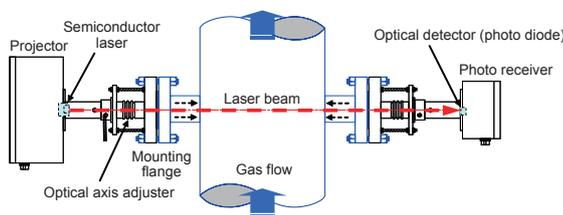
**Figure 3** Measurement of Flue Gas Concentration by the TDLS200
