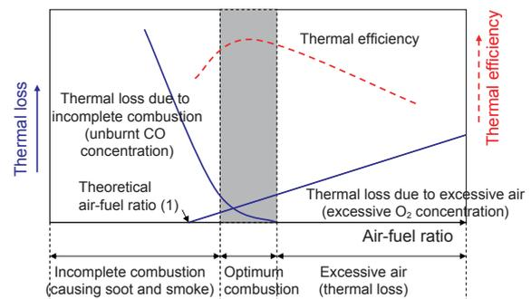
**Figure 1** Relationship between Air-fuel Ratio and Heat Efficiency (Combustion)
