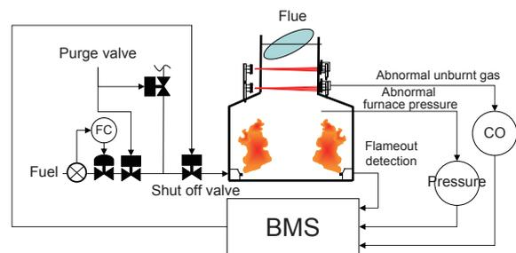
Figure 6 Safety Control in the Burner Control Equipment
