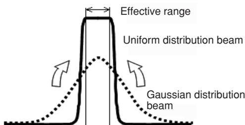
**Figure 7** Adjustment of the Intensity Distribution in the Laser Beam
