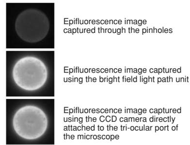
**Figure 11** Image Captured Using the Bright Field Light Path Unit
