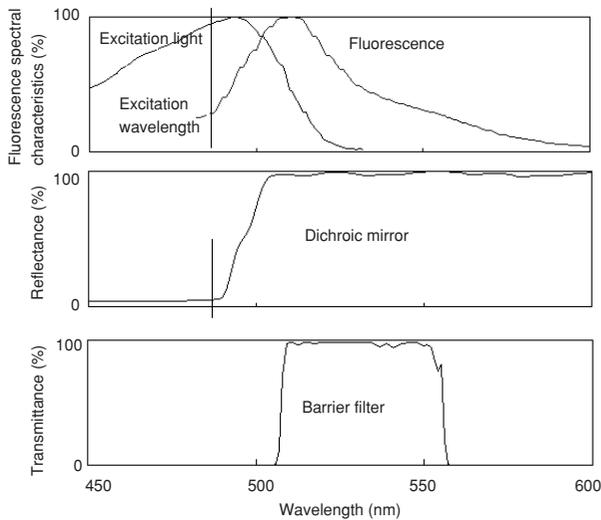
**Figure 9** Example Spectral Characteristics of a Filter
