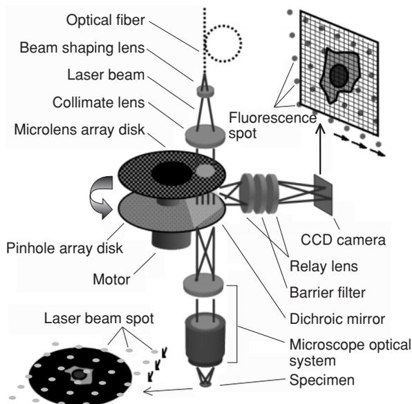
**Figure 5** Configuration of the Optical System Used in the CSU-X1
