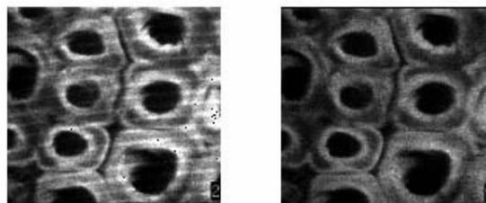
**Figure 8** Suppression of Stripes by Adjusting Rotation Speed; stripes due to the fraction of time (left)/no stripes because an integral multiple is met (right)
