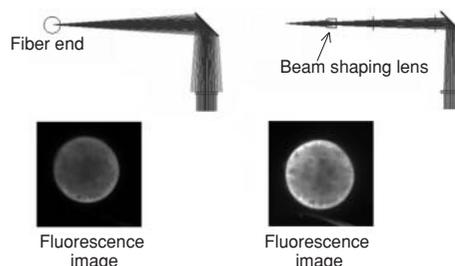
**Figure 6** Intensity Distributions of the Laser Beam; an image captured using a conventional technique (left) and an image improved by using a beam shaping lens
