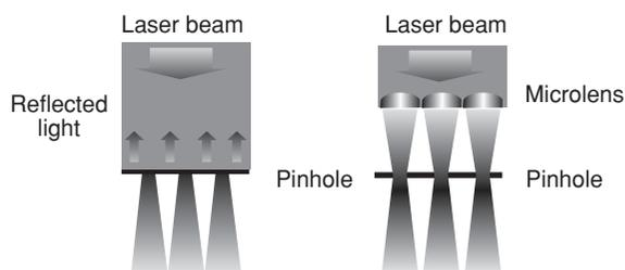
**Figure 4** Improvement in Optical Characteristics Resulting from the Use of Microlenses; the backscattering light remains (left) and increase in the amount of the laser light passing through the pinholes (right)
