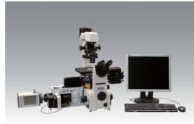
**Figure 13** An Example System Configuration of a Confocal Microscope
