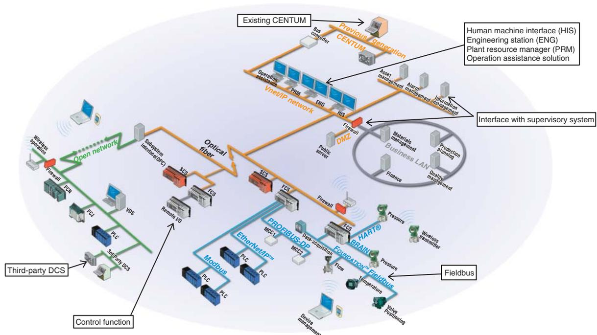
**Figure 4** Configuration Example of Process Control System Using CENTUM VP
