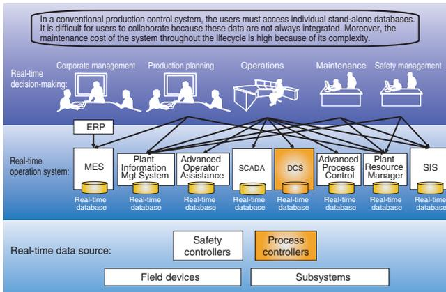
**Figure 2** Functions of Conventional DCSs
