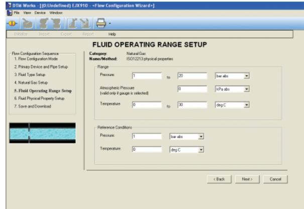
**Figure 4** Mass Flow Calculation Setup Operation Screen on the EJX910DTM
