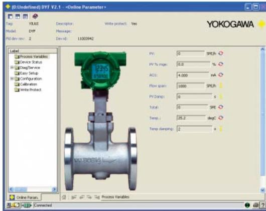
**Figure 3** Device DTM Online Parameter Function GUI (Example)
