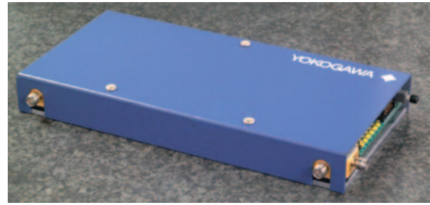
Figure 2 CDR Subsystem (200 × 100 × 24.2 mm)
