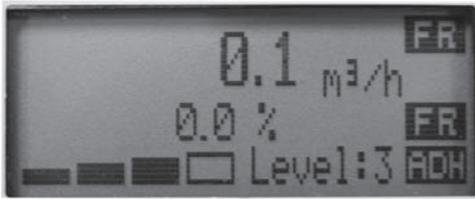
Figure 14 Example of Adhesion Level Display
