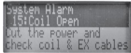
**Figure 20** Alarm Display Mode
