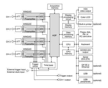
Figure 2 DL1600 Block Diagram
