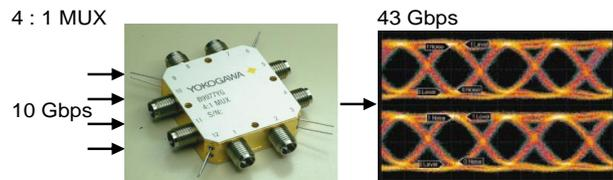
**Figure 15** 43-Gbps,  $2^{31}-1$  PRBS Output Waveform of 4:1 MUX IC Module (Amplitude: 0.5 Vpp)
