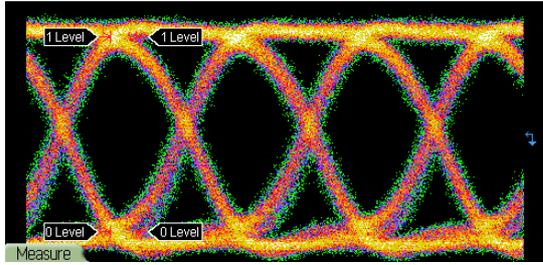
**Figure 6** Output Waveform (Containing 1.1-ps Jitter) of Optical Modulator Driver-IC Module with 40-Gbps,  $2^{31}-1$  PRBS Input Data
