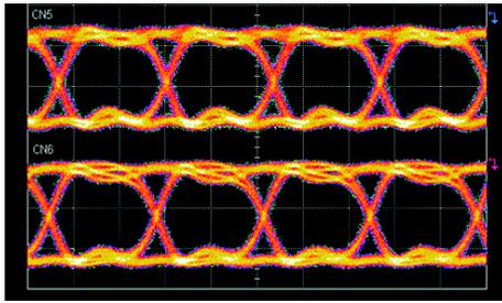
**Figure 11** Output Waveforms of 1:2 DEMUX IC Module with 43-Gbps,  $2^{31}-1$  PRBS Input Data
