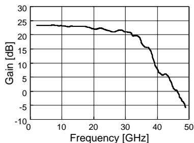
**Figure 4** Frequency-gain Characteristics of Optical Modulator Driver-IC Module
