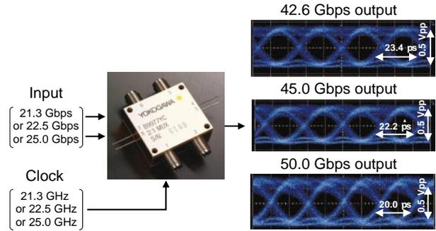
**Figure 9** Output Waveforms of 2:1 MUX IC Module with  $2^{31}-1$  PRBS Input Data
