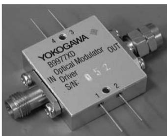
**Figure 3** Optical Modulator Driver-IC Module
