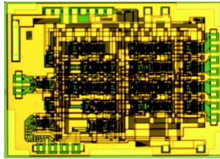
**Figure 14** 1:4 DEMUX IC Module Chip (43-Gbps,  $2.8 \times 3.8$ mm, 3.2 W, 1600 Circuit Elements Integrated)
