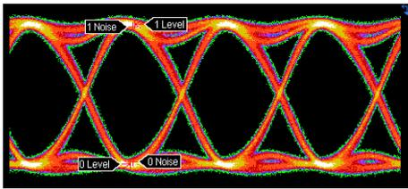
**Figure 12** Output Waveforms of DFF IC Module with 43-Gbps,  $2^{31}-1$  PRBS Input Data
