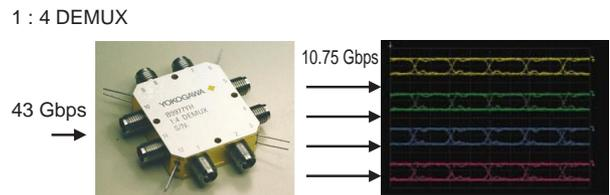
**Figure 16**  $2^{31}-1$  PRBS Output Waveforms of 1:4 DEMUX IC Module with 43-Gbps Inputs (Amplitude: 0.5 Vpp)
