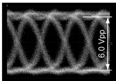
**Figure 5** Output Waveform of Optical Modulator Driver-IC Module with 43-Gbps,  $2^{31}-1$  PRBS Input Data
