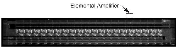
**Figure 2** IC Chip of Twenty-stage Cascade Distributed Amplifier
