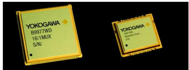
**Figure 20** Ceramic-packaged 16:1 MUX and Optical Modulator Driver IC Modules
