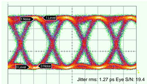
**Figure 7** Output Waveform of LN Optical Modulator (supplied by Sumitomo Osaka Cement Co., Ltd.) with 43-Gbps,  $2^{31}-1$  PRBS Input Data
