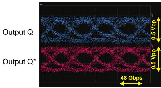
**Figure 17** 48-Gbps Output Waveforms of 4:1 MUX IC in the on-wafer state
