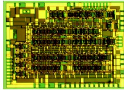
**Figure 13** 4:1 MUX IC Module Chip (43-Gbps,  $2.8 \times 3.8$  mm, 3.5 W, 2000 Circuit Elements Integrated)
