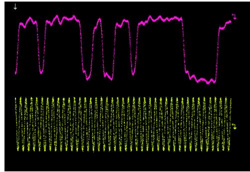
**Figure 23** Output Data Waveform and Clock Waveform of CDR
