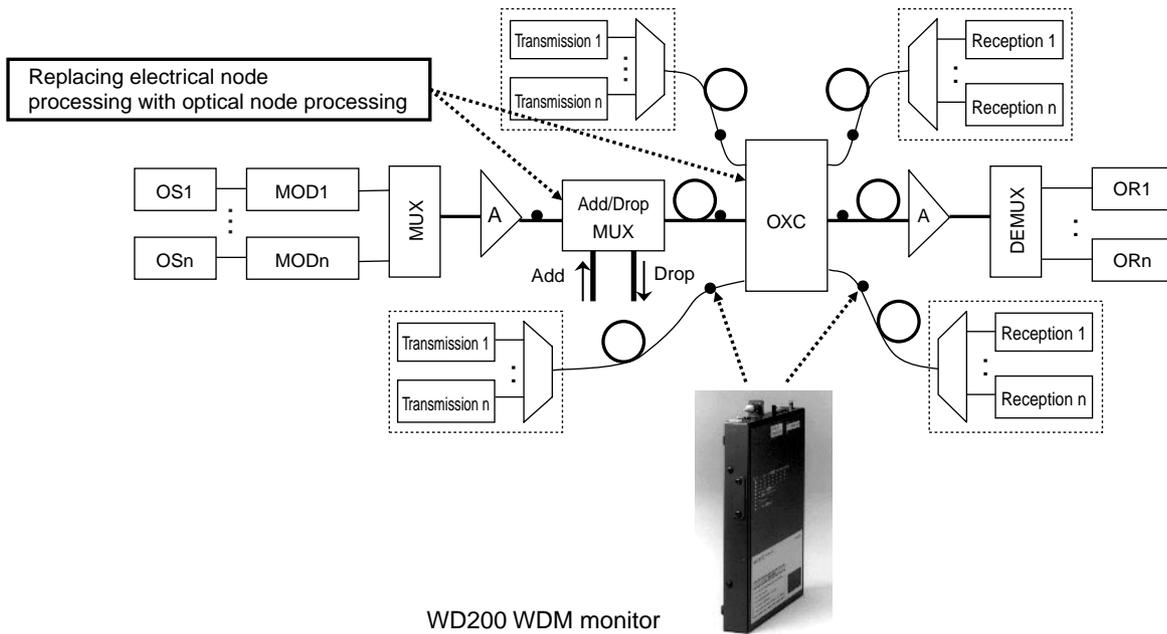
**Figure 1** Networking WDM Systems and WDM Monitors
