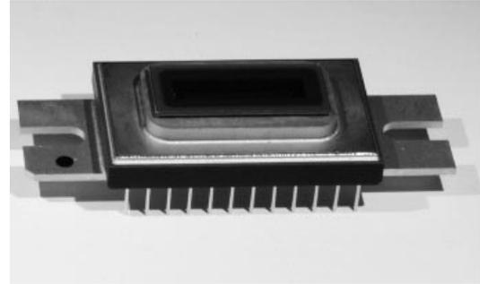
**Figure 5** 640-pixel InGaAs PDA
