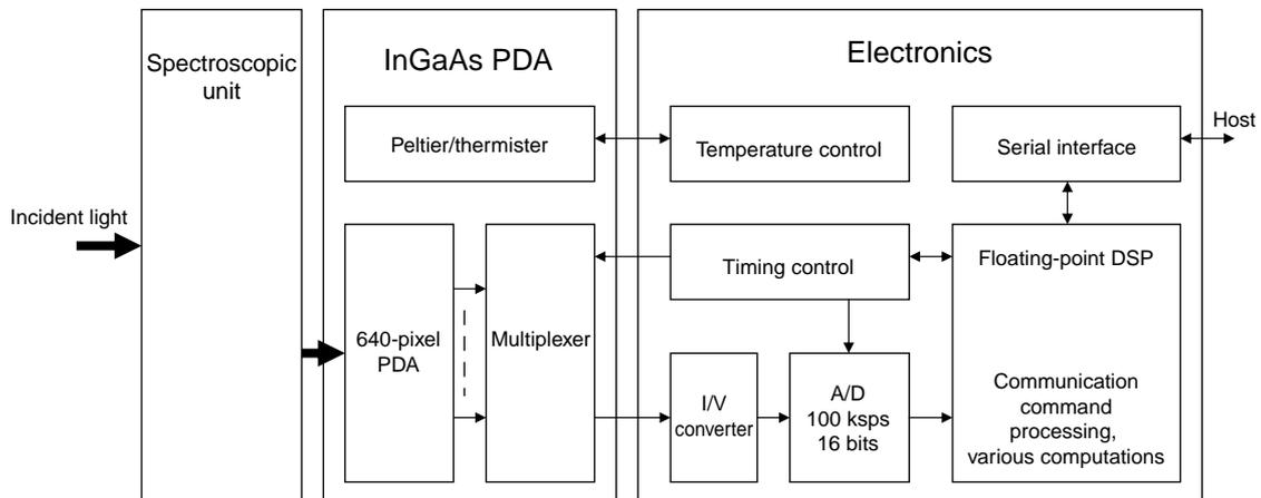
**Figure 2** WD200 Block Diagram
