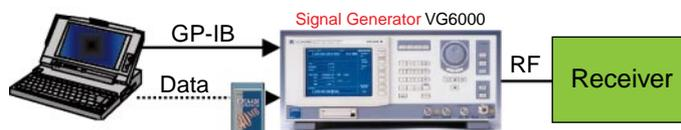
**Figure 1** Receiver Performance Test System
