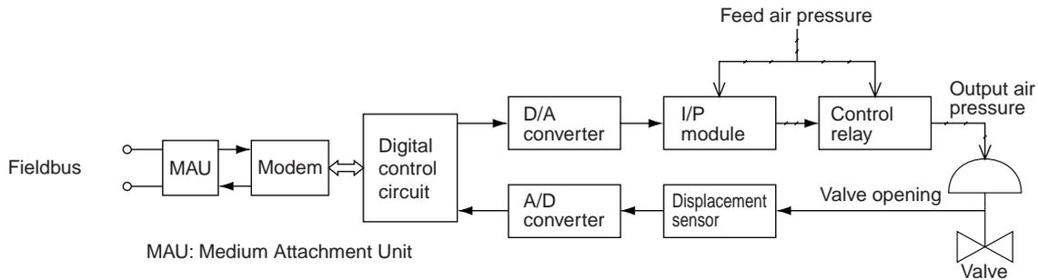
**Figure 2** Block Diagram of YVP110
