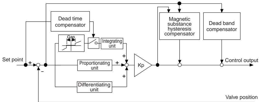
**Figure 3** Block Diagram of PID Control with Nonlinearity Compensation
