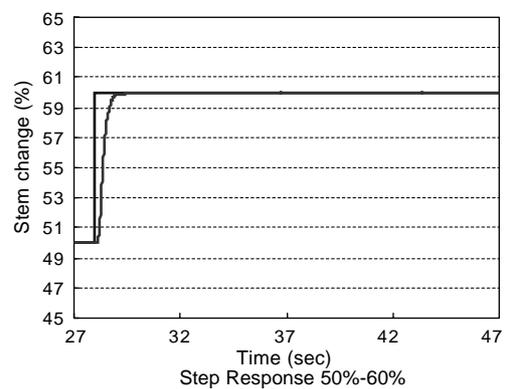
**Figure 5** Response Characteristics of PID Control with Nonlinear Compensation
