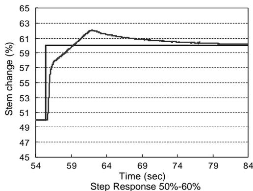
**Figure 4** Response Characteristics of Normal PID Control
