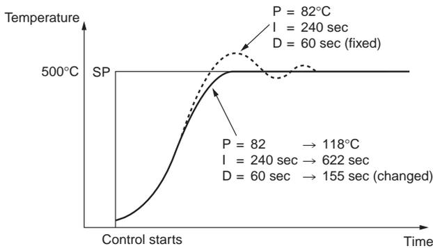
**Figure 5** When Controller Starts Up
