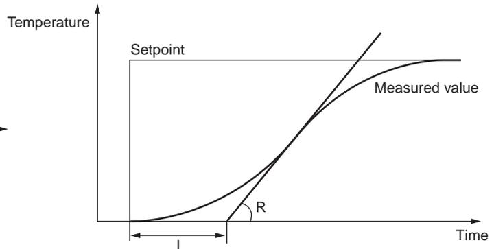
**Figure 3** Calculation of PID Values at Controller Startup
