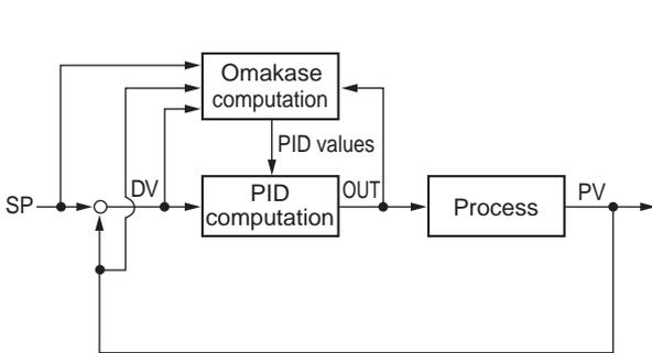
**Figure 2** Block Diagram of Omakase Control
