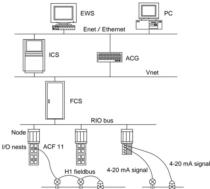
**Figure 1** CENTUM CS System Configuration
