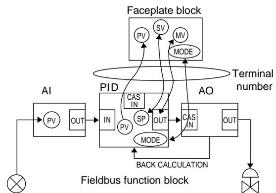
**Figure 4** Operation and Monitoring Using a Faceplate Block
