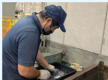
Checking for foreign matter using magnets
