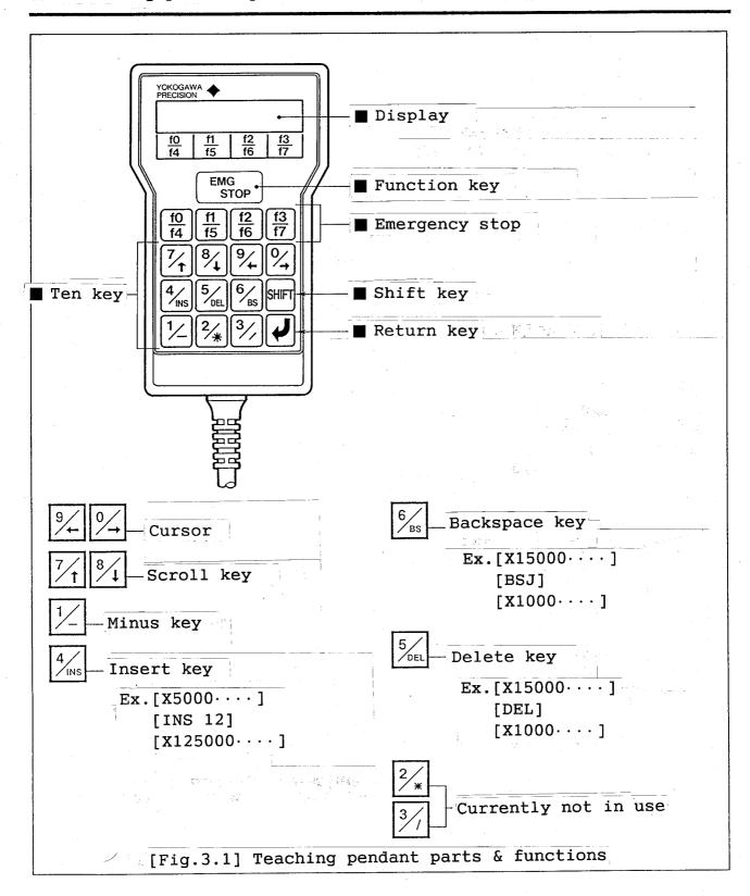
Items indicated in the display screen sequentially starts with the opening screen, followed by direct input screen(No.1-2 menu screen), Program parameter input screen(No.3 menu screen), and the edit screen(No.4 menu)
