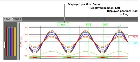
If you left-click the mark while pressing the "Ctrl" key, the mark is displayed in front. If you left-click the mark while pressing the "Shift" key, the mark is displayed in the back. Double-clicking a mark, that has been created using the Data Viewer, opens the [Mark] dialog box in which you can change the displayed group and the mark name.
