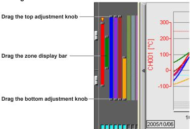
You can change the waveform display zone on the waveform display screen by clicking the edit zone icon on the tool bar or by selecting [Y-Axis] - [Edit Zone] in the menu bar. The size of the zone can be changed by dragging the top and bottom adjustment knobs. The entire zone can be moved by dragging the zone display bar.
