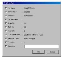
The items that are checked are output in the header when printed.
