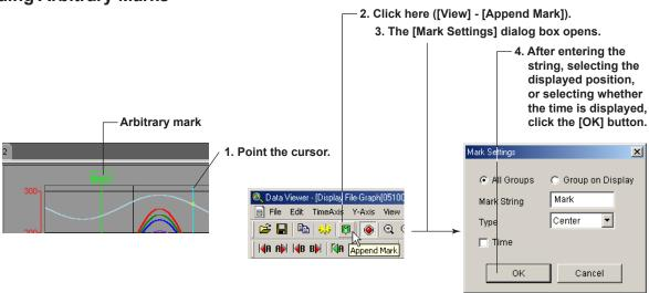
When Cursor A and Cursor B are at the same position, arbitrary marks can be placed. You can select whether to put the arbitrary marks on all groups or only on the displayed group. And you can set the displayed position of the mark and select whether the time is displayed by the mark.
