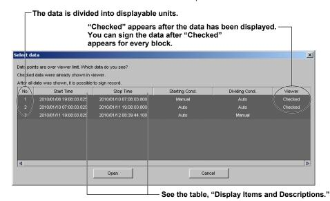
To sign into a batch file that contains 5 million data points or more, first put all the files in the batch in a single folder, and then open all the files from the Select data dialog box. While you are opening divisions, do not move files, delete them, or perform other file operations.
