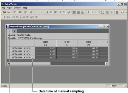
If a file contains manually sampled data that has been acquired under different conditions, they are displayed separately using tabs.
