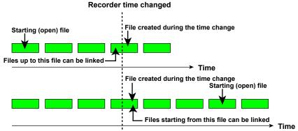
· The linked data display is based on the time of the starting file.
