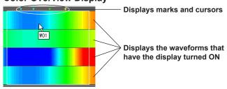
The measured values of the entire data are displayed using various colors. By assigning 50 different colors from the minimum to the maximum values of the scale, the measured values are assigned to those colors.
