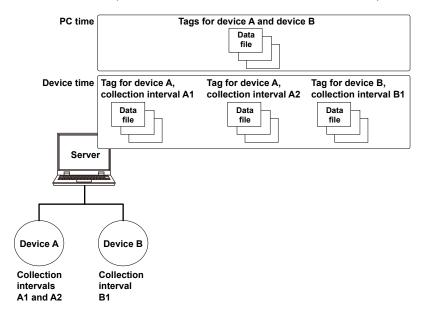
The device number, device name, and device acquisition interval are included in the names of data files. Below is the file name format when date and time are included. FileName-DeviceNo-DeviceName-Interval-YYYYMMDDhhmmss.ext
