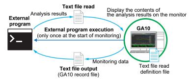
The external access function is only enabled if the data time is PC time. The function is disabled for Device time and does not operate.
