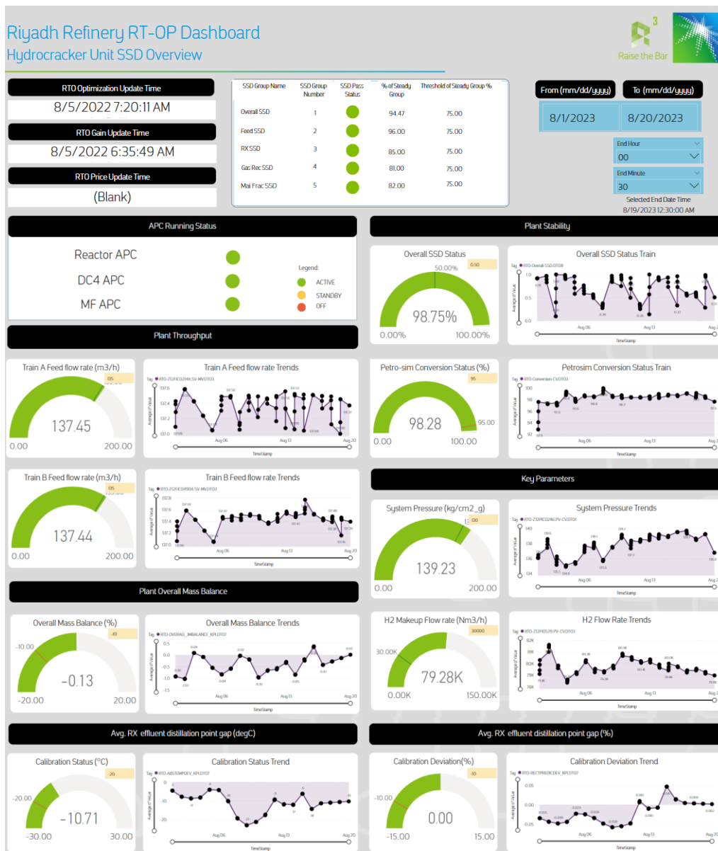
Figure-07- Yokogawa RT-OP dashboard
