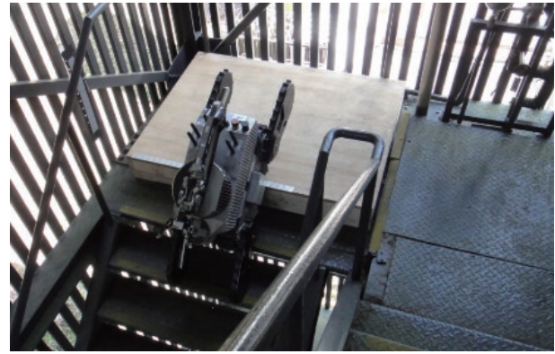
Figure 7 Wooden base installed at an obstacle location on the test route
