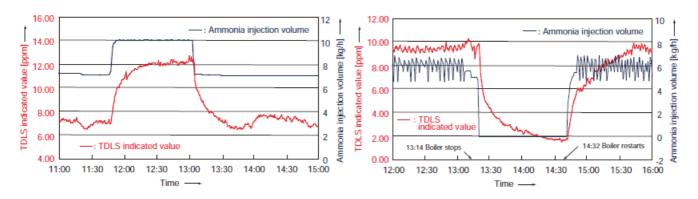
The TDLS responds to  $NH_3$  injection volume changes at high speed and thus is able to control and monitor the optimum  $NH_3$  injection volume.
