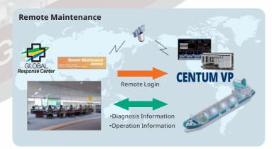
Yokogawa service engineer can remotely log in to onboard CENTUM via VSAT. The operator can make immediate and precise action with Yokogawa consultation. Safest security measures are built-in to the onboard connection.
