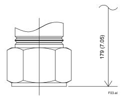
• Process Connections: 1/2 NPT male (Process Connection Code 7)
