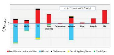
Figure 3: Carbon Dioxide uses, costs, and margins
