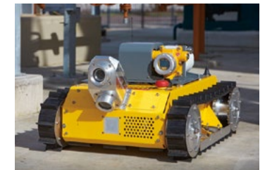
ExRobotics' robot for inspection tasks: ExR-1
