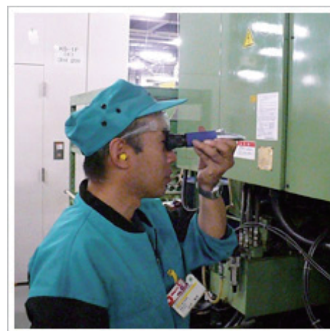
Using Refractometer to Check the Density of Cutting Fluid
