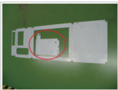
Different parts are punched out from off-cuts.
