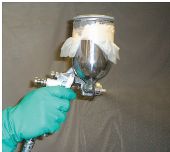
Sprayer for Low-Toluene/Low-Xylene Polyester Paint
