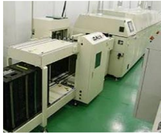
Nitrogen reflow oven with lead-free soldering process installed in the surface mount line
