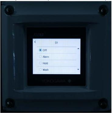
Once an item is selected, the analyzer will return to the previous screen. The save icon  $\blacksquare$  in the top right must be pressed for any changes to be stored.
