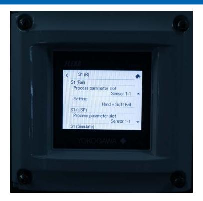
Be sure to press  $\blacksquare$  to store any changes before exiting the contact option page. For additional details on each option refer to section 4.4 in the FLXA404 operation manual Operation Manual
