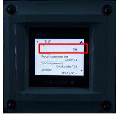
Options for S1, S2, and S3 include Alarm, Hold, Wash, Error, USP, Simulate, and Off. S4 options include Alarm, Error, Simulate, and Fail safe. For a full description of each option, see Chapter 4.4 in the FLXA402 Operation Manual.
