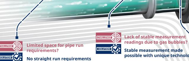
The Rotamass TI Hygienic model is not affected by flow velocity distribution due to its unique measurement principle. Therefore, upstream/downstream pipe runs are not required.
