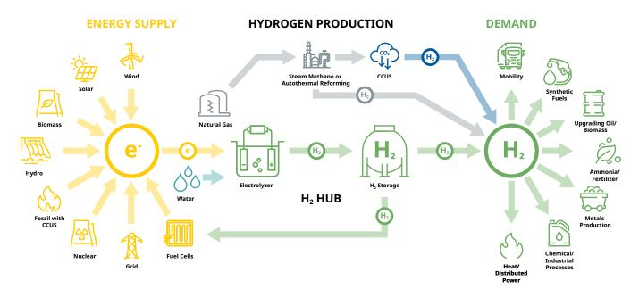
The hydrogen industry used to be about process units such as electrolyzers and reformers. Now, it is an emerging ecosystem complete with hydrogen hubs, power grids, and a broad consumer base.
