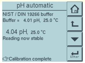
11.) To have the analyzer finish and accept calibration data press the diamond next to Accept Data
