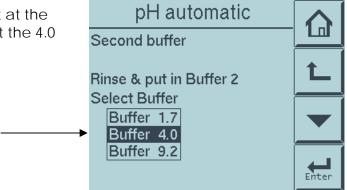
9.) The main display will start flashing and continues to flash until the reading has stabilized for 5 seconds and does not change by more than .02 pH units.
