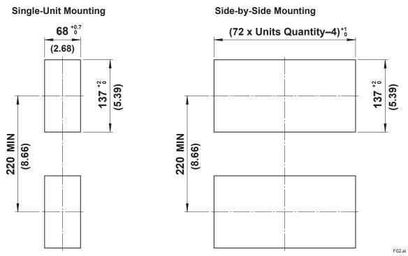
Note: If not specified, the tolerance is ±3%. However, for dimensions less than 10 mm, the tolerance is ±0.3 mm.
