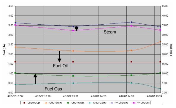
Boiler D (FO and FG): 2 t/h less of steam) and FO to the minimum
