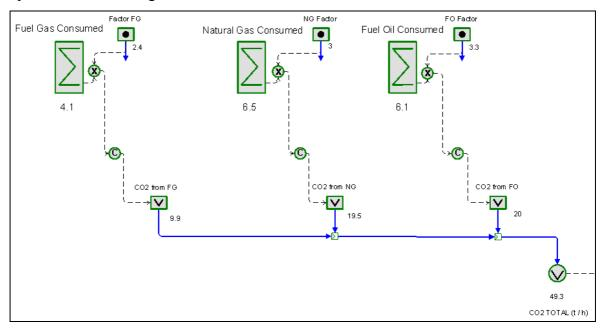
*Figure 3.* Details of the  $CO_2$  emissions model differentiated by the type of Fuel
