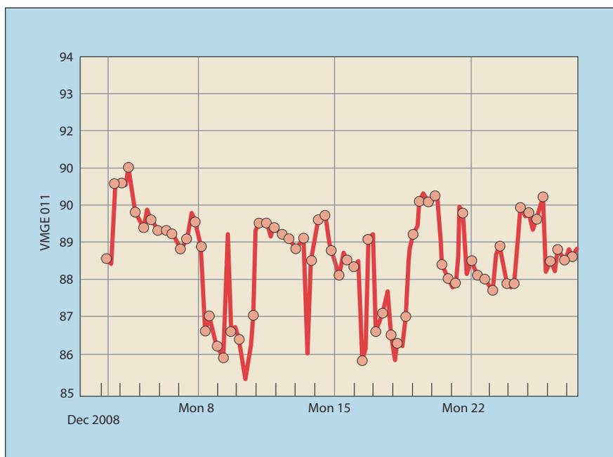
Figure 3 Boiler efficiency trend
