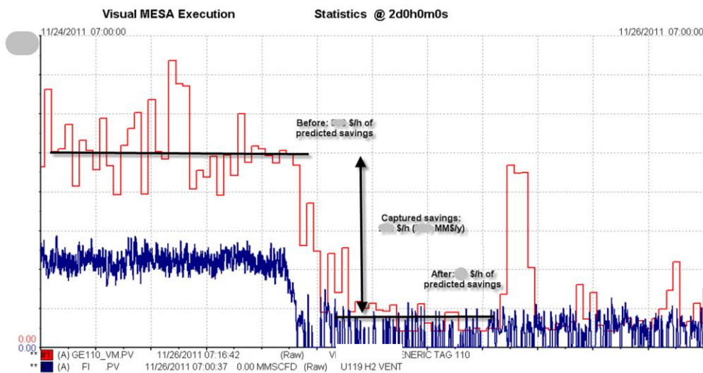
Figure 10 – Total savings, in $/h, captured after the closing of the hydrogen vent in one of the Units
