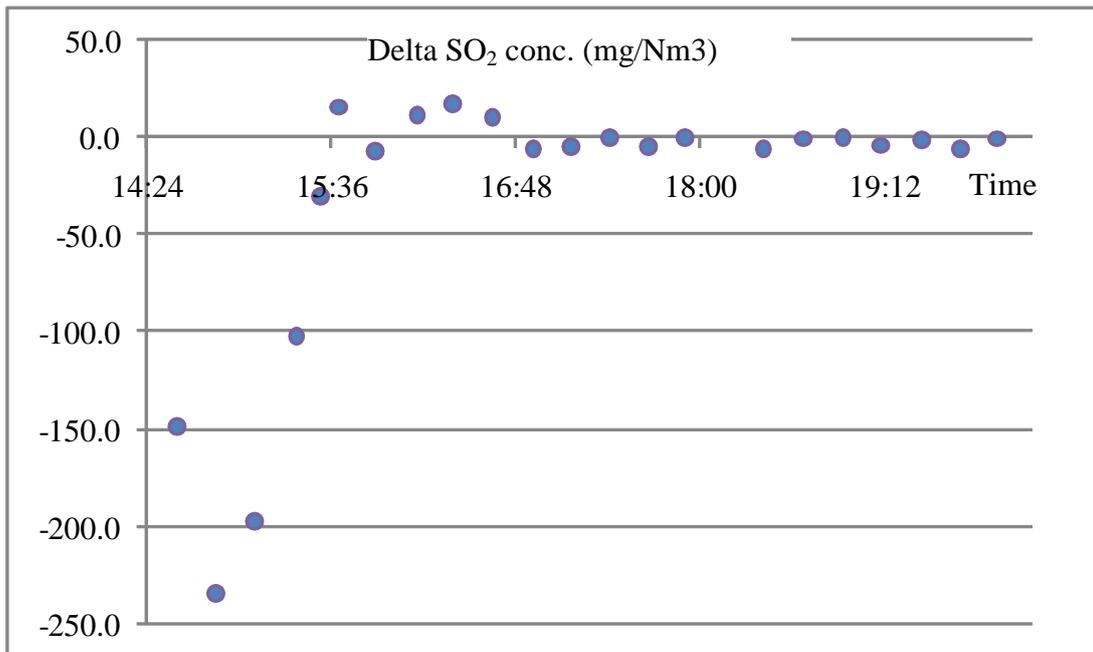
Figure 3. Identified SO<sub>2</sub> emissions reduction along a shift
