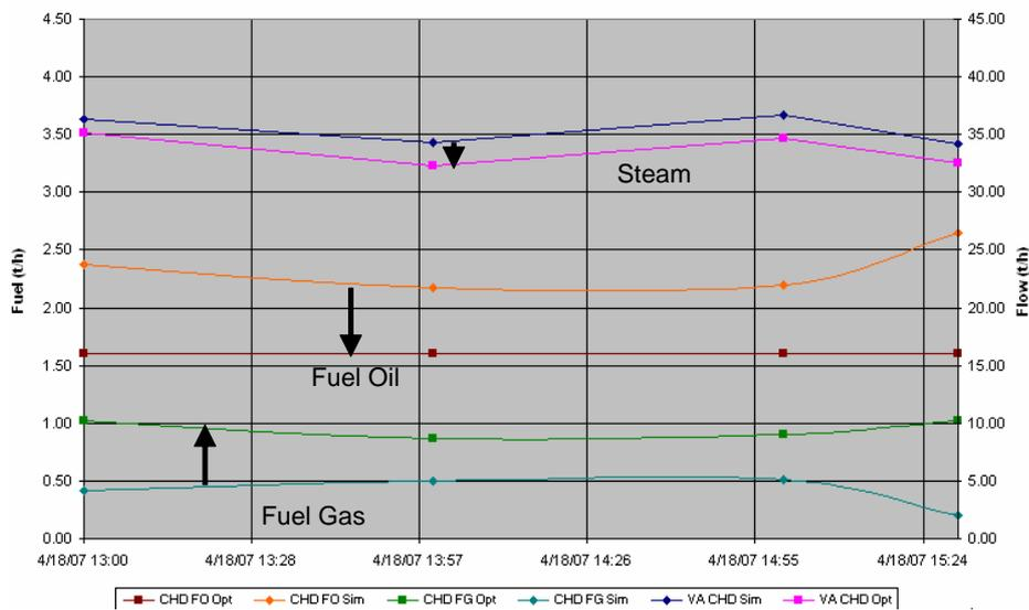
Figure 13. Boiler D (FO and FG): steam production reduced 2 t/h and FO reaching the minimum constraint
