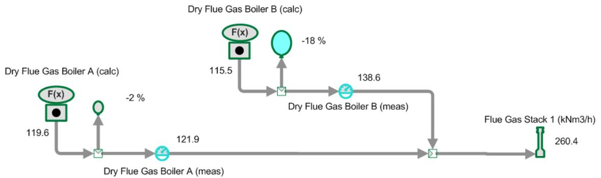
Figure 4b. Flue gas flow calculation.
