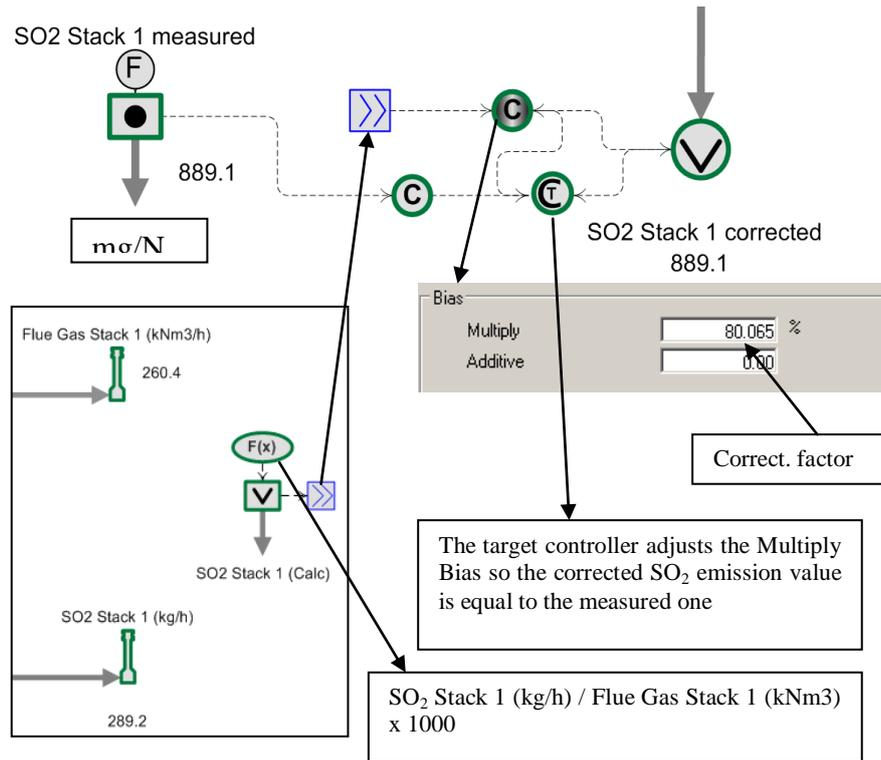
Figure 4c. SO<sub>2</sub> model calculation biasing when concentration is measured
