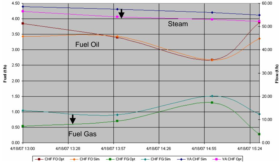
**Figure 14. Boiler F (FO and FG): steam production reduced more than 3 t/h**
