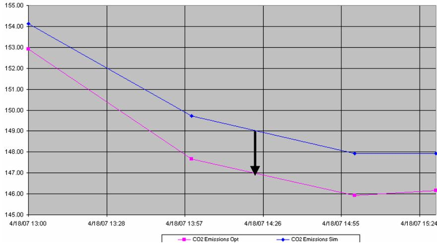
**Figure 15. Overall CO<sub>2</sub> emissions reduced 2 t/h**
