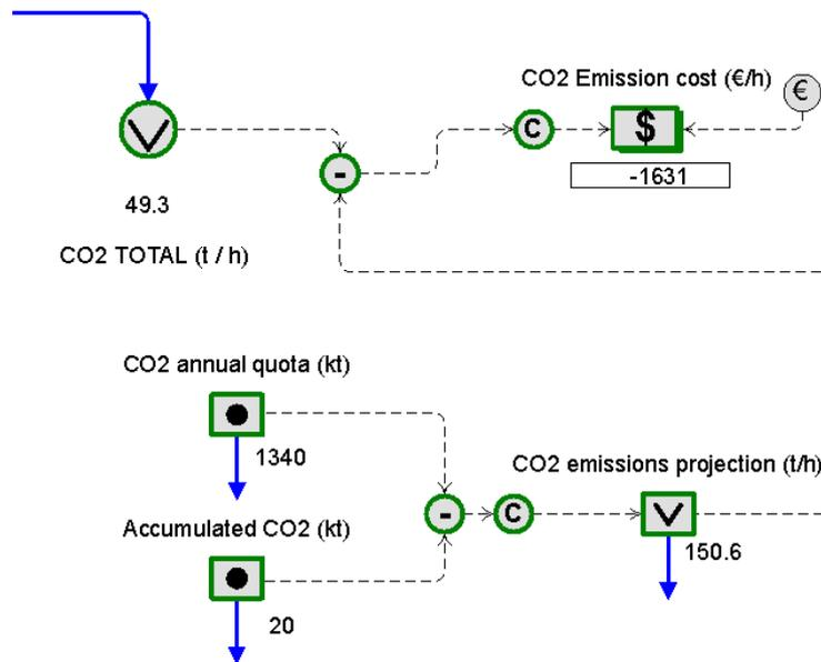
Figure 9. CO<sub>2</sub> cost based on projected emission
