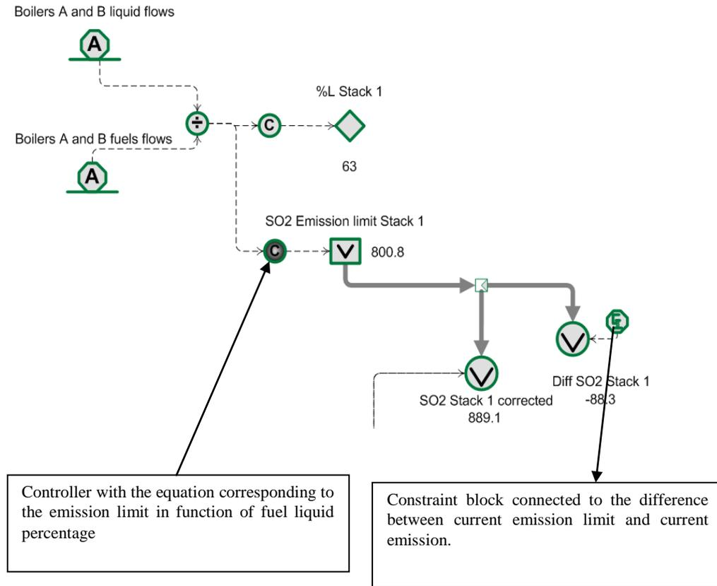
Figure 4d. SO<sub>2</sub> model emission limit and constraint.
