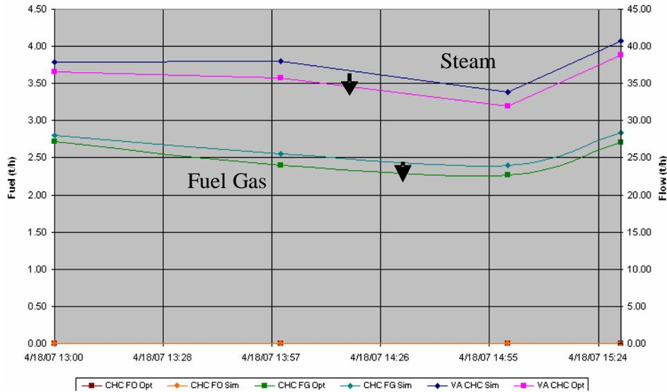
Figure 12. Boiler C (100% Fuel Gas): steam production reduced 2 t/h
