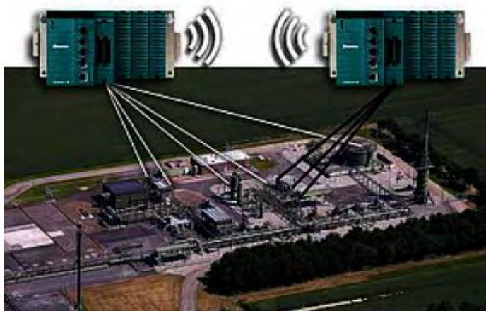
Figure 6. Remote condition and performance monitoring for large pieces of critical equipment by the OEM already is happening. The result is often multiple SCADA systems working in parallel at the same site. The way these systems interact must be carefully controlled.
